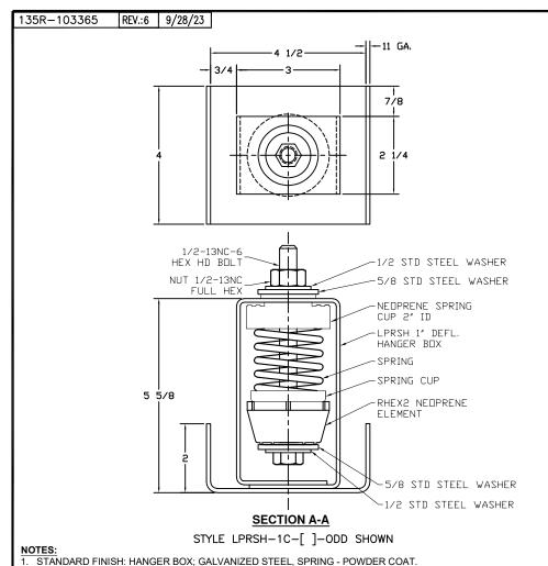
MODEL LPRSH-1C ELASTOMERIC & SPRING HANGER 1" DEFLECTION **RATED** RATED LOAD SPRING RATE **COLOR** DEFLECTION **HANGER** (LBS) (LBS/IN) CODE (IN) LPRSH-1C-15 15 1.00 15 DK. GRAY LPRSH-1C-25 25 1.00 25 GREEN LPRSH-1C-50 50 1.00 50 BLUE LPRSH-1C-100 100 1.00 100 TAN LPRSH-1C-150 150 1.00 RED 150 LPRSH-1C-250 250 0.83 300 BLACK LPRSH-1C-300 DK YELLOW 300 0.75 400
